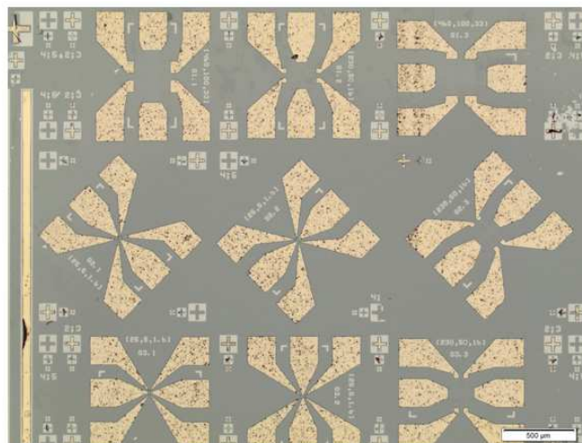
Fig. 5.11 Hall bars fabricated on 1LG sample by lithography technique developed in L2C.
