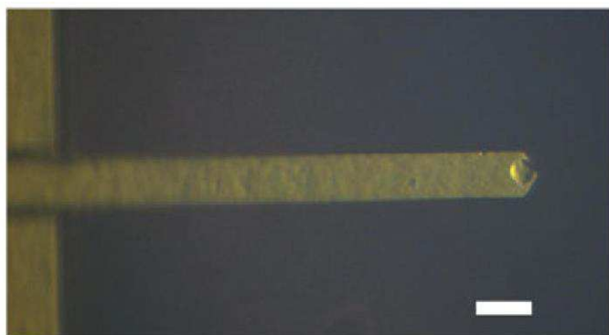
FIGURE 3 Bottom view of a tumor cell immobilized at the end of an atomic force microscope cantilever (scale bar is 50 \mu\text{m} )
