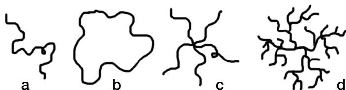
Figure 8 – Example of polymers with different structures: linear (a), ring (b), star (c), randomly branched (d).
