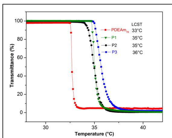
**Figure 4** Transmittance (%) of solutions of PDEAm (red), **P1** (green), **P2** (black) and **P3** (blue) in 0.2 % (w/v) in respect to temperatures (0.2 °C min<sup>-1</sup>).
