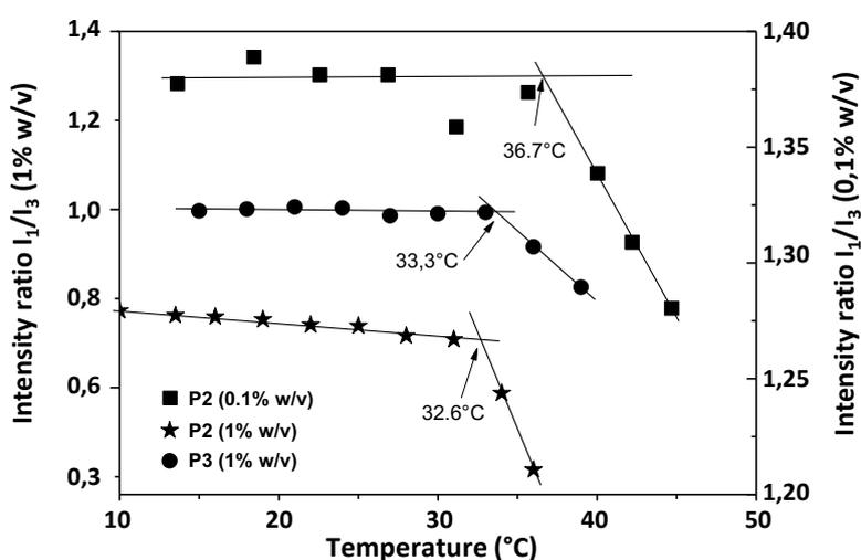
**Figure 6** Temperature dependence of the fluorescence intensity ratio  $I_1/I_3$ . **P2** (0.1% w/v) (square); **P2** (1% w/v) (star) and **P3** (1% w/v) (circle). [Pyrene] =  $2 \cdot 10^{-6}$ M.
