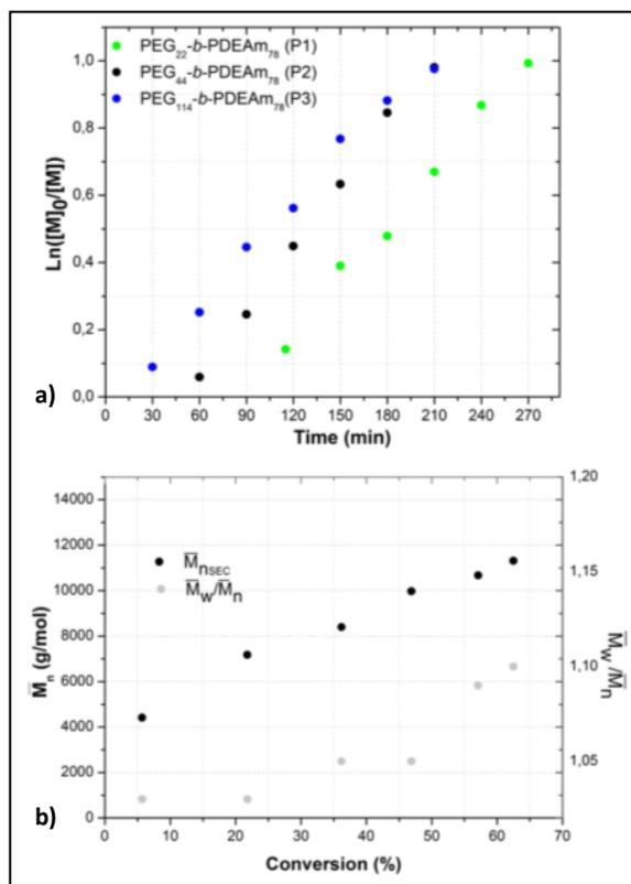
**Figure 2** a) First-order kinetic plots of DEAm polymerizations with PEG macro-CTAs of different chain lengths (750 (P1), 1900 (P2) and 5000 (P3) g mol<sup>-1</sup>) in dioxane at 80 °C. [Monomer]:[macro-CTA]:[AIBN]= 672:6:1. b) Evolution of  $M_n$  vs. monomer conversion for the polymerization of DEAm initiated by PEG<sub>44</sub> macro-CTA 1900 g mol<sup>-1</sup> (P2).
