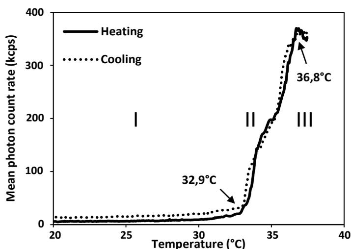
**Figure 7** Plot of the mean photon count rate of a 0.1 % w/v solution of **P2** vs. temperature (heating/cooling rates = 0.2 °C min<sup>-1</sup>).
