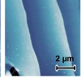
Steps width increases with lowering the temperature ramp
