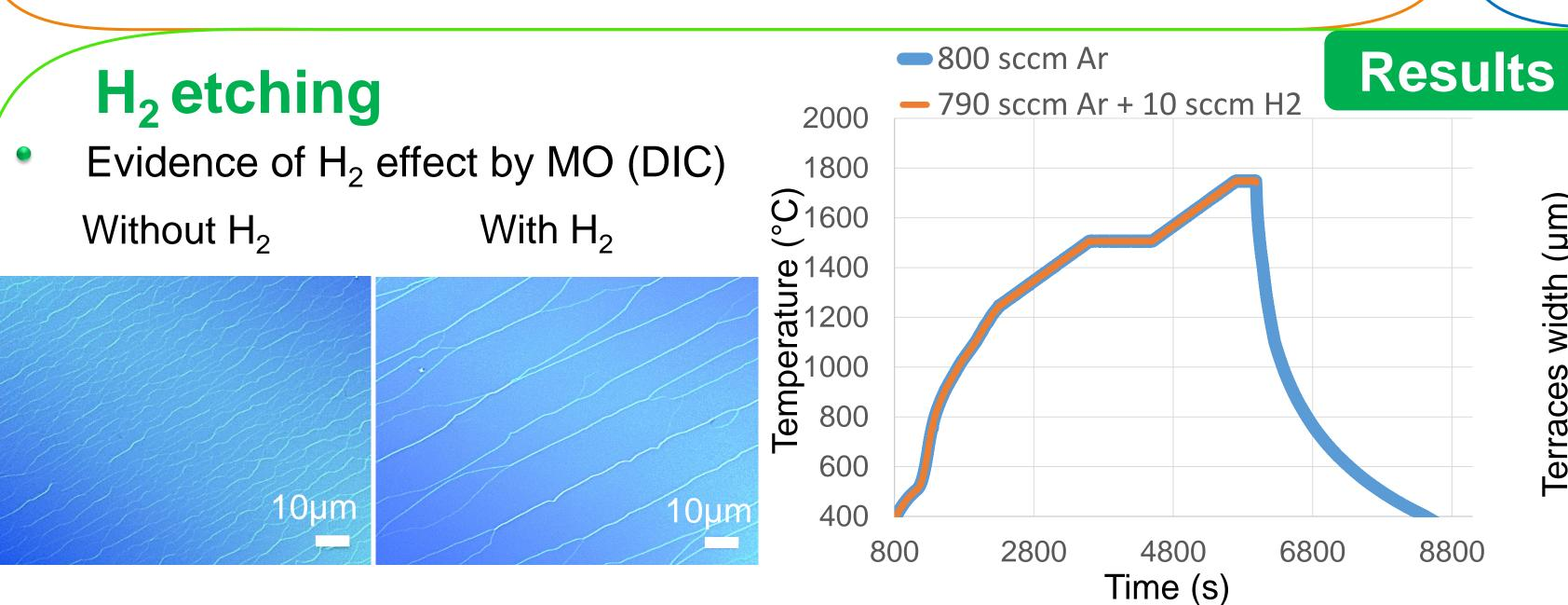
Large terraces up to 15 µm with H<sub>2</sub> covered with buffer layer
