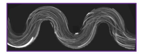
The experimental study is performed for a dilute polymer solution in a wavy microchannel. The channel of width W comprises a series of half loops of radius R which is systematically varied. We have analyzed the critical Weissenberg number ( $Wi_c$ ) at which the flow becomes unstable as a function of the geometry of the channel and the properties of the polymer solution.
